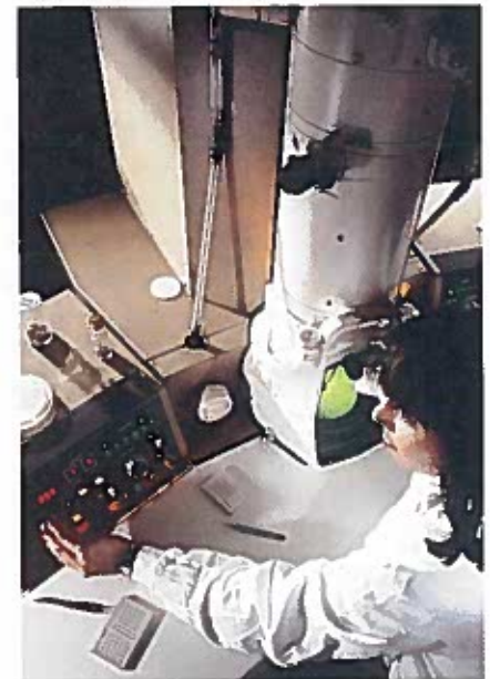
B Transmission electron microscope (TEM). Electrons passing through a thin slice of a specimen illuminate a fluorescent screen. Internal details of the specimen cast visible shadows, as in Figure 4.8d.
